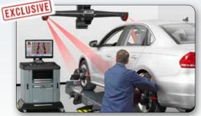
Compensate all wheels and capture initial measurements in one motion
